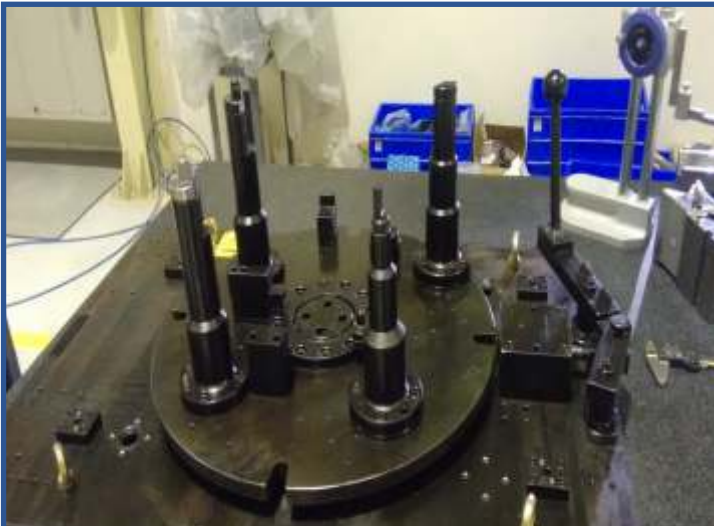
Assembly Fixture For Hub Of Axle For Tata Motors
