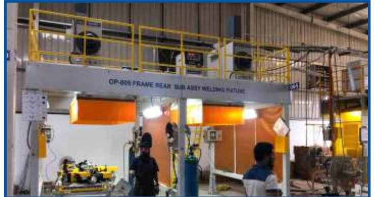
Electro pneumatic Welding cell station
