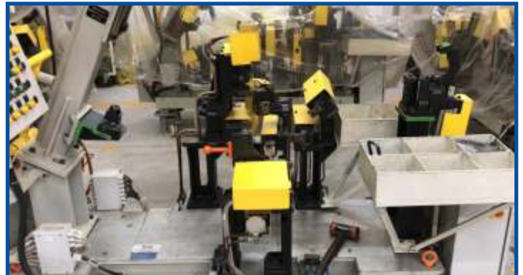
Electro pneumatic welding fixture for Upper tube ,TVS
