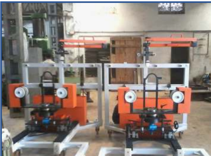
Lifting & Sliding Mechanism For Assembly Of Caterpillar Gear Box
