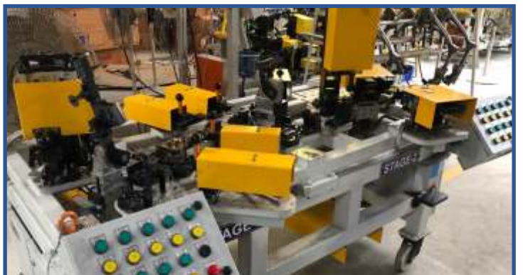
Electro pneumatic welding fixture for Side Tube ,TVS
