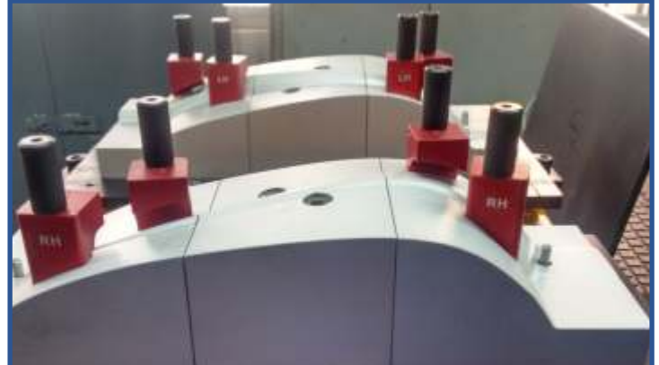
Checking fixture for side view mirror cover ,Toyota Etios
