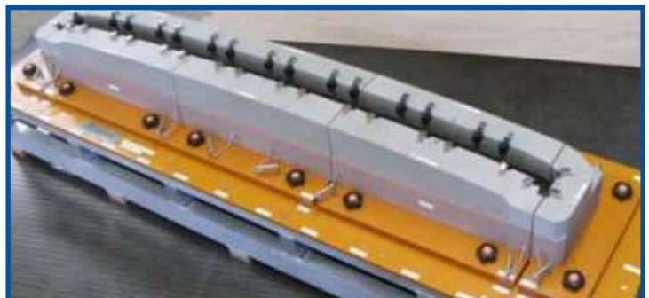
Gauge for part checking ,Toyota Gosei
