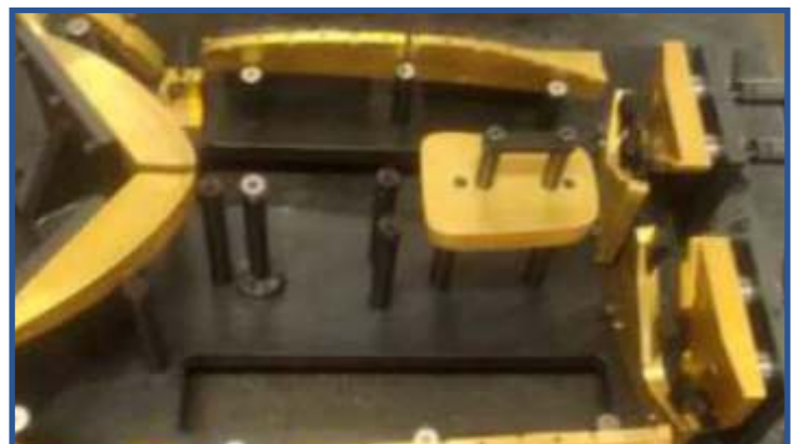
Checking fixture for Floor bound panel , TVS Scooter
