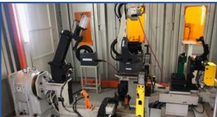
Robotic welding fixture for 2 Wheeler Frame
