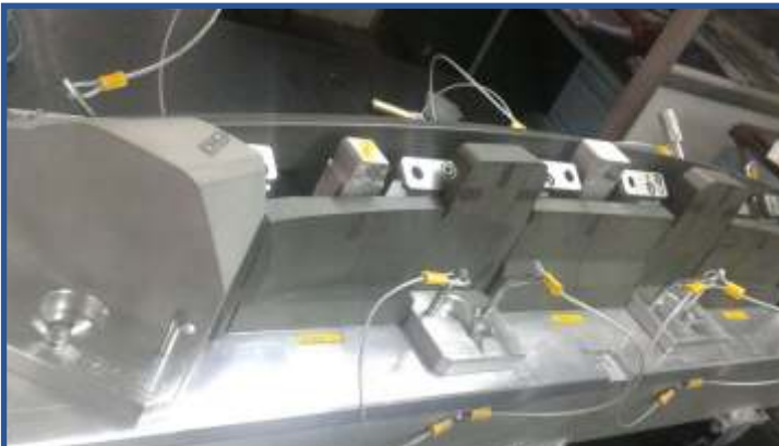
Checking fixture for Front panel , Toyota Etios
