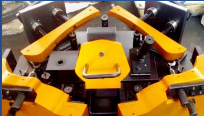
Checking fixture for Speedometer Console ,TVS Scooter
